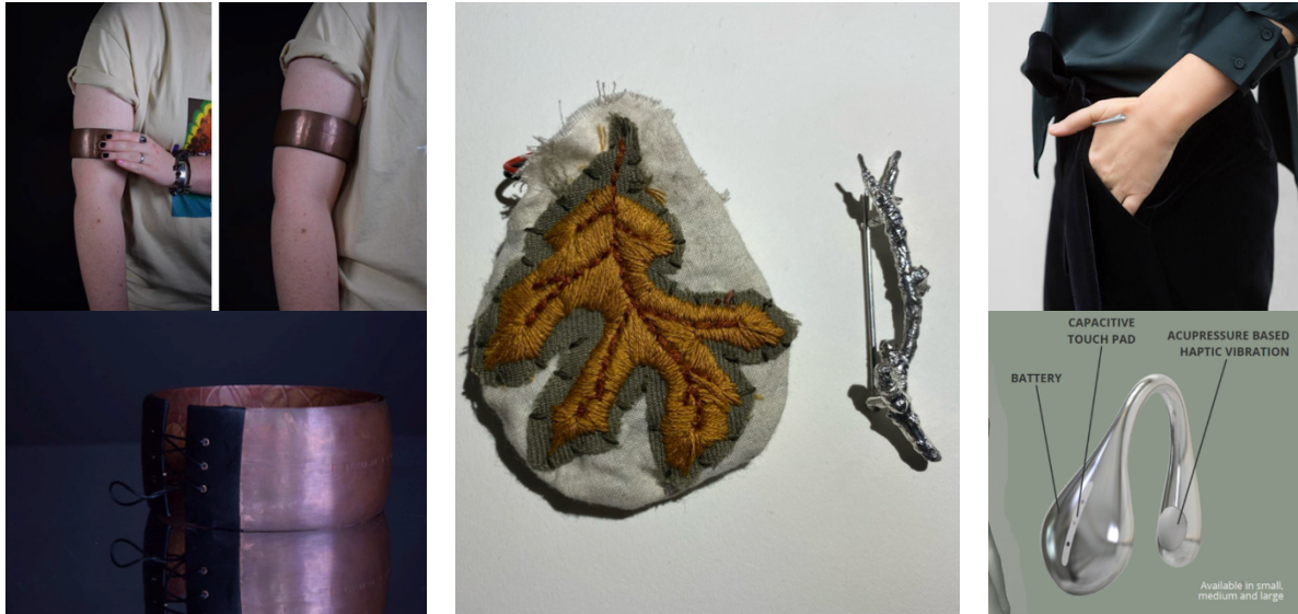
Figure 7 (left to right) a) Amulet for Anxiety : (top) The wearer touches the piece to activate the vibration. (bottom) Detail of the leather section that can be manually tightened. middle b) Nature : Detail of the embroidered bag that houses the electronics and the silver twig-shaped brooch. c) Alleviate : (top) Worn between the thumb and index finger, (bottom) showing a visual description of the electronic components.
