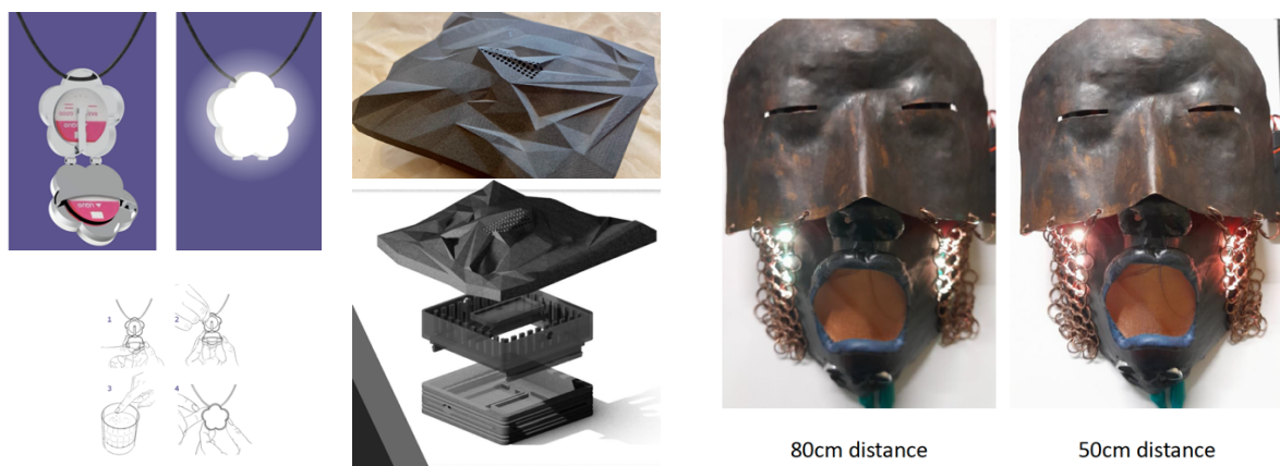
Figure 9 (left to right) a) Bloomtech: Visual representation of the piece and its use b) Withdrawn: The 3D-printed piece alongside a 3D visualisation of its interior. c) Mask: Light projections showing distance cues: green at 80 cm, red at 50 cm.
